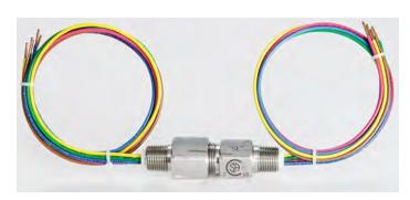
When HL Fittings are supplied with factory-installed wires from Conax, the fittings are factory torqued. A bar is laser engraved across the Body and Cap to allow user to verify that the fitting is still properly torqued.
