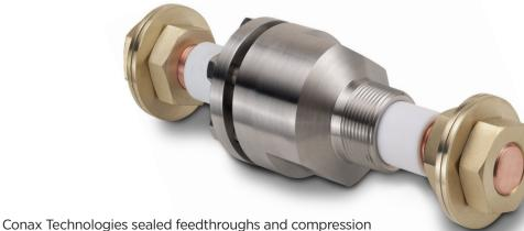
seal fittings have proven to be the industry leaders in quality and performance. We are the originators of soft sealant technology that, when combined with mechanical compression, results in a remarkably secure and leak tight seal on wires, probes, and electrodes passing through a pressure or environmental boundary.
