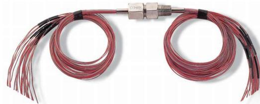
These feedthrough assemblies comprise a high-density, wire feedthrough mounted in a seal fitting. A PTFE-lined, stainless steel tube is swaged over 12, 24, 40 or 60 solid, PTFE-coated, copper and/or thermocouple material wires to make the high-density continuous wire feedthrough for thermocouples, RTDs and low voltage instrumentation.
