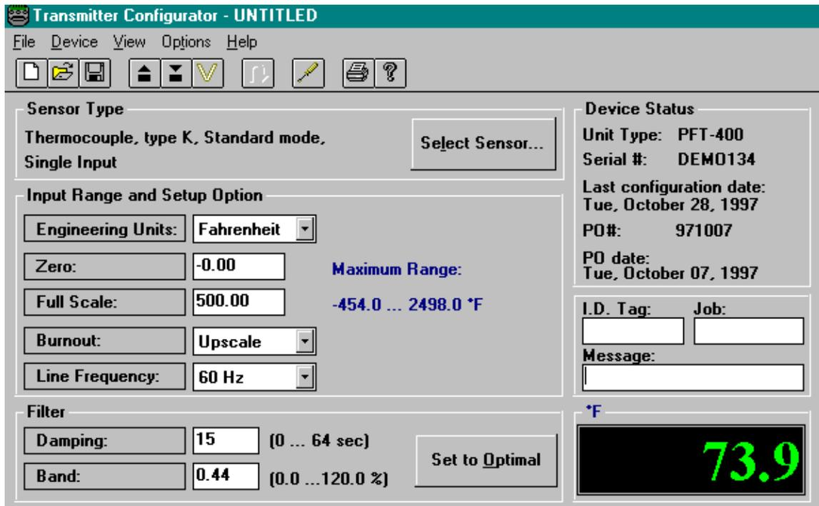
7.2.5 Select the input sensor type by clicking on the “**Select Sensor**”
