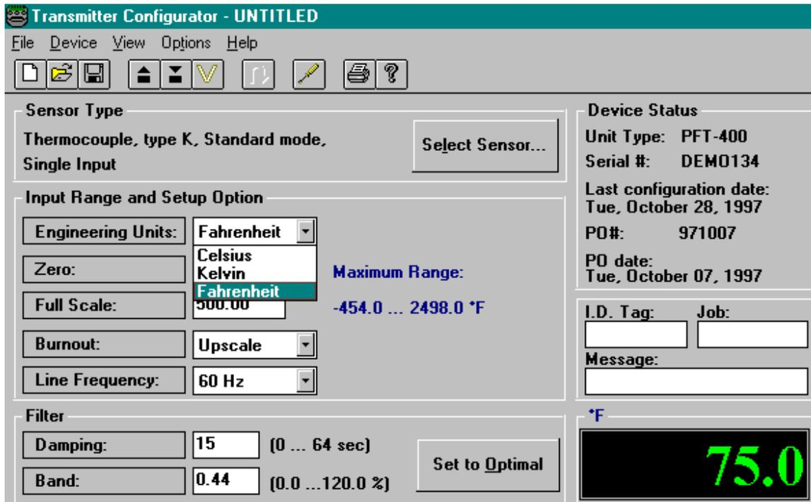
7.2.8 TAB down to the next box which is “Zero”. Just to the right of the “Zero” box in blue type is the maximum allowable measurement range for the selected sensor. Enter the “Zero” value to define the specific low input range. Next TAB down to the “Full Scale”. Enter the “Full Scale” value that defines the transmitters high input range. (See Figure 8)
