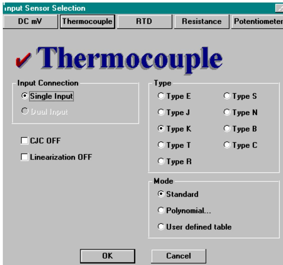
7.2.6 Click on the various selection boxes which best define your sensor’s parameters. Click the **OK** button to return to the main screen. On the main screen next to the “**Select Sensor**” box, you will see the **Sensor Type** that has been selected (See Figure 6). This is to confirm the selection made on the previous screen.
