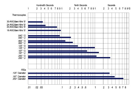
In determining time constants for the bar charts above, tests were performed in still water going through an instantaneous step change from 32°F to 212°F.
