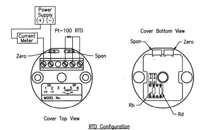
Note: For a 2 wire RTD hookup, a jumper wire must be installed between terminals 4 and 5.
