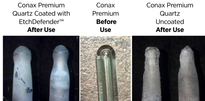
Figure 1. (left) Image of 2 EtchDefender™ TCs run at a Fab in an ASM Epsilon® reactor. (center) Example of the Standard quartz sheath before population with the thermoelements and prior to running in the reactor. (right) Image of 2 Standard TCs run at the same Fab to failure under identical process parameters.
