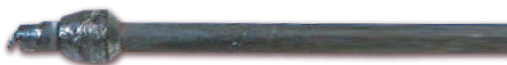
Standard exhaust gas sensor after vibrations have caused the tip to break and sensor to fail.
