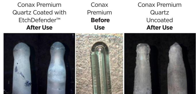
Figure 1. (left) Image of 2 EtchDefender<sup>™</sup> TCs run at a Fab in an ASM® EPSILON® Reactor. (center) Example of the Standard quartz sheath before population with the thermoelements and prior to running in the reactor. (right) Image of 2 Standard TCs run at the same Fab to failure under identical process parameters.
