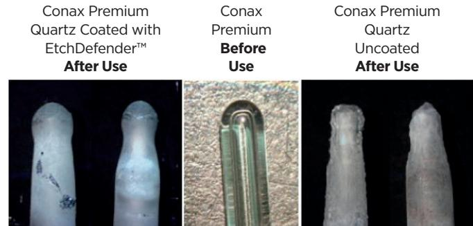
Figure 1. (left) Image of 2 EtchDefender<sup>™</sup> TCs run at a Fab in an ASM Epsilon<sup>®</sup> reactor. (center) Example of the Standard quartz sheath before population with the thermoelements and prior to running in the reactor. (right) Image of 2 Standard TCs run at the same Fab to failure under identical process parameters.
