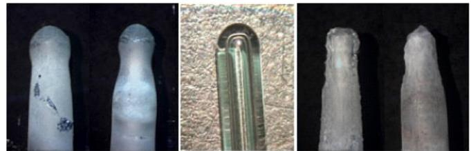
Figure 1. (left) Image of 2 EtchDefender<sup>™</sup> TCs run at a Fab in an ASM<sup>®</sup> EPSILON<sup>®</sup> Reactor. (center) Example of the Conax uncoated premium quartz sheath before population with the thermoelements and prior to running in the reactor. (right) Image of 2 uncoated TCs run at the same Fab to failure under identical process parameters.
