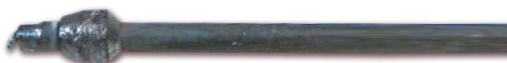
Standard exhaust gas sensor after vibrations have caused the tip to break and sensor to fail.
