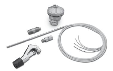
Trimmable RTDs provide versatility, accuracy and ease of use in one rugged unit, with a 4-wire lead configuration that provides measurements of the highest precision. The trimmable RTD's easy, cut-to-fit feature allows the user to alter the length of the RTD sheath to fit into various thermowells, pipewells and tubewells. The stainless steel sheath is trimmable, using a commercially available tube cutter, down to a length of 6" (15.2cm).
