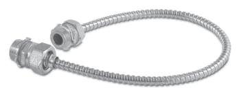
Conax Flex-Tube Assemblies protect wires from mechanical abuse. They are available in any length, factory assembled and furnished complete with end fittings (standard male or female pipe thread). Standard end fittings are plated brass or steel. Stainless steel Conax Compression Seal Fittings (PG) may be substituted at additional cost.
