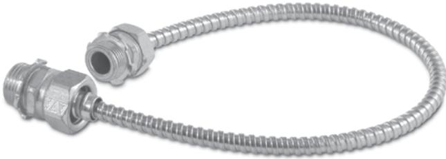
Conax Flex-Tube Assemblies protect wires from mechanical abuse. They are available in any length, factory assembled and furnished complete with end fittings (standard male or female pipe thread). Standard end fittings are plated brass or steel. Stainless steel Conax Compression Seal Fittings (PG) may be substituted at additional cost.
