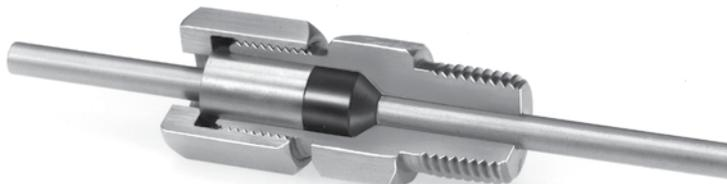
This stainless steel, single bore compression seal fitting seals sheathed thermocouples, RTDs or other probes against gases or liquids. Conax “soft sealant” technology uses a compressible material, allowing the seal to be untorqued to adjust the probe immersion, then retorqued to re-establish the seal.
