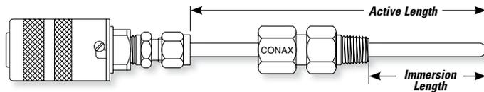
When ordering spring loads, the immersion length should be measured with the spring uncompressed. We recommend 1/4" of spring compression when the probe is installed.
