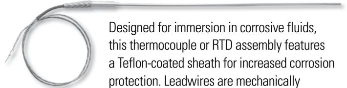
Designed for immersion in corrosive fluids, this thermocouple or RTD assembly features a Teflon-coated sheath for increased corrosion protection. Leadwires are mechanically protected by a stainless steel braid (T4). The assembly is normally terminated with a Conax PJ male plug. Teflon coating can be applied to most sensor probe assemblies presented in this catalog.
