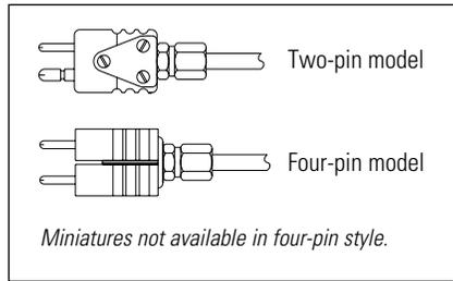
Conax B-Series heads are compact, lightweight terminal heads that provide convenient hook-up of customer extension wire. The cap and body are nickel-plated to resist corrosion. The ceramic terminal block contains zinc-plated brass terminal posts that accept up to 14 AWG wire. Bayonet-style cover allows easy access to the terminal posts. B-Series heads are provided in direct or adjustable mounting styles.
