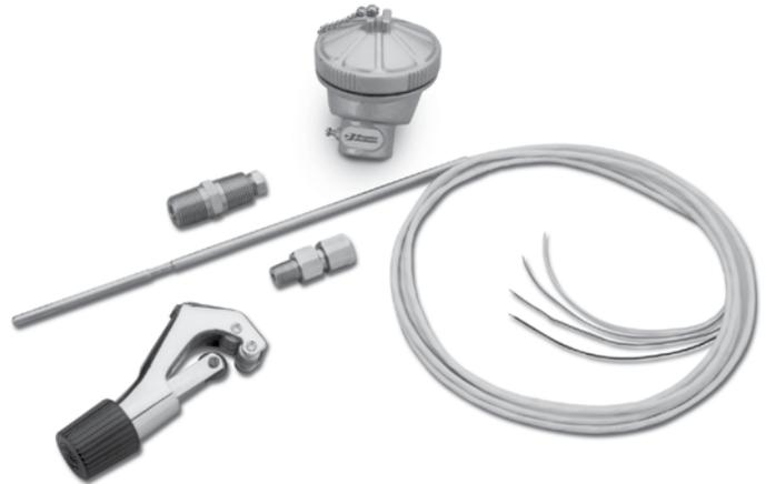
Trimable RTDs provide versatility, accuracy and ease of use in one rugged unit, with a 4-wire lead configuration that provides measurements of the highest precision. The trimmable RTD's easy, cut-to-fit feature allows the user to alter the length of the RTD sheath to fit into various thermowells, pipewells and tubewells. The stainless steel sheath is trimmable, using a commercially available tube cutter, down to a length of 6" (15.2cm).
