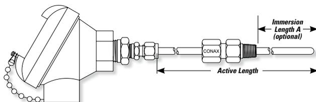
With adjustable fittings and spring-load assemblies, the immersion length is measured from the end of the fitting to the tip of the probe. In cases where this length must be called out in the catalog description, it is added at the end of the catalog number as follows:
