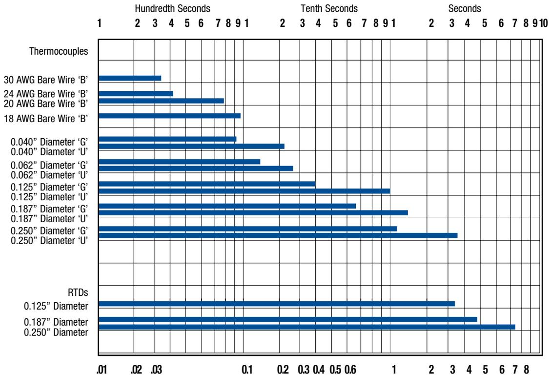
In determining time constants for the bar charts above, tests were performed in still water going through an instantaneous step change from 32°F to 212°F (0°C to 100°C).
