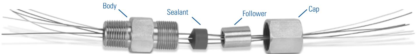
Conax BSWS assemblies were originally designed for use with embedment bearing temperature sensors to prevent oil migrating along the sensor leads. They seal on the individual insulated leads exiting an oil-filled bearing house. They may also be used to seal all types of insulated instrumentation lead wire. These sealing assemblies can be found in large motors, generators, turbines, pumps, compressors and journal bearing pedestals.
