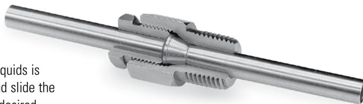
This all stainless steel assembly for sealing gases and liquids is easy to use. Simply open the compression seal fitting and slide the assembled fitting over the tube or probe. Tighten at the desired location. The ferrule is deformed against the probe and makes a seal without cutting the sheath surface.
