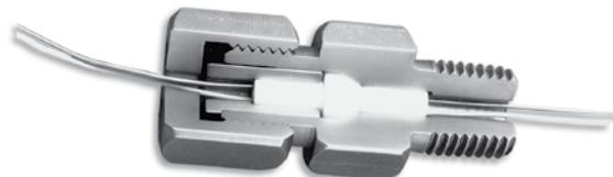
This assembly consists of a Conax Technologies manufactured instrumentation wire feedthrough (TG) with a Teflon or Grafoil sealant and Teflon-coated thermocouple grade or copper wires. Typical applications include the sealing of wires exiting compressor bearing housings, pressure vessels, instruments, furnaces and reactors. The compression seal is furnished with 24" (61cm) of wire on each side. Longer wire lengths can be furnished as required.
